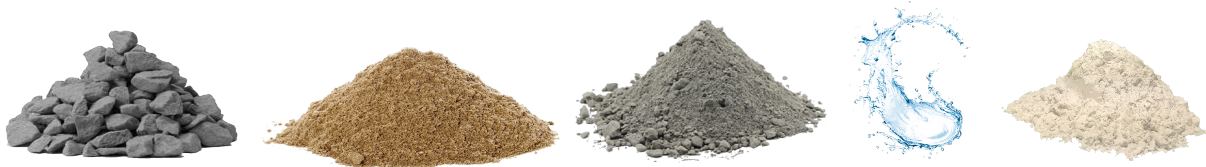
The components of concrete (L to R), gravel, sand, cement, water, and pantheon™.
